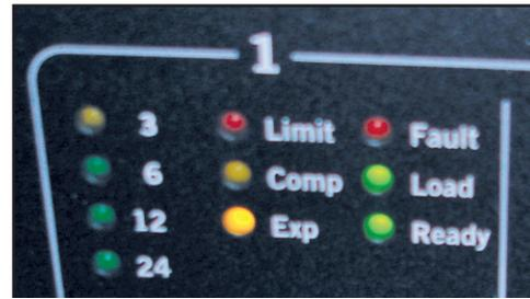
The Rane MA 4 Amplifier has a "Load" light that is "off" if the load exceeds 16 ohms, "on" if between 2 and 16 ohms, and "flashes" if the load is less than 2 ohms. This alerts the user that they are excessively loading the amplifier.
